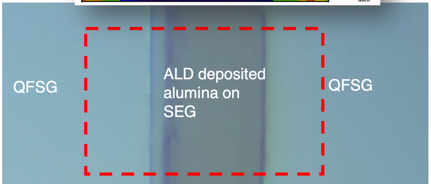
Extended Data Fig. 7 | Example of a seamless SEG/QFSG junction. The junction was produced by depositing an \text{Al}_2\text{O}_3 strip, 80 \mu\text{m} wide, and intercalating hydrogen at 700 C.
