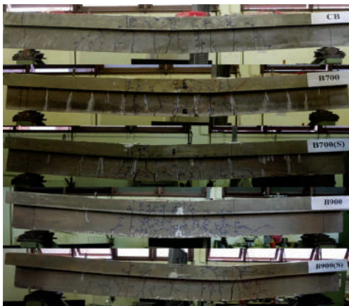
Fig. 8—Failure and crack patterns of RC T-beams.
