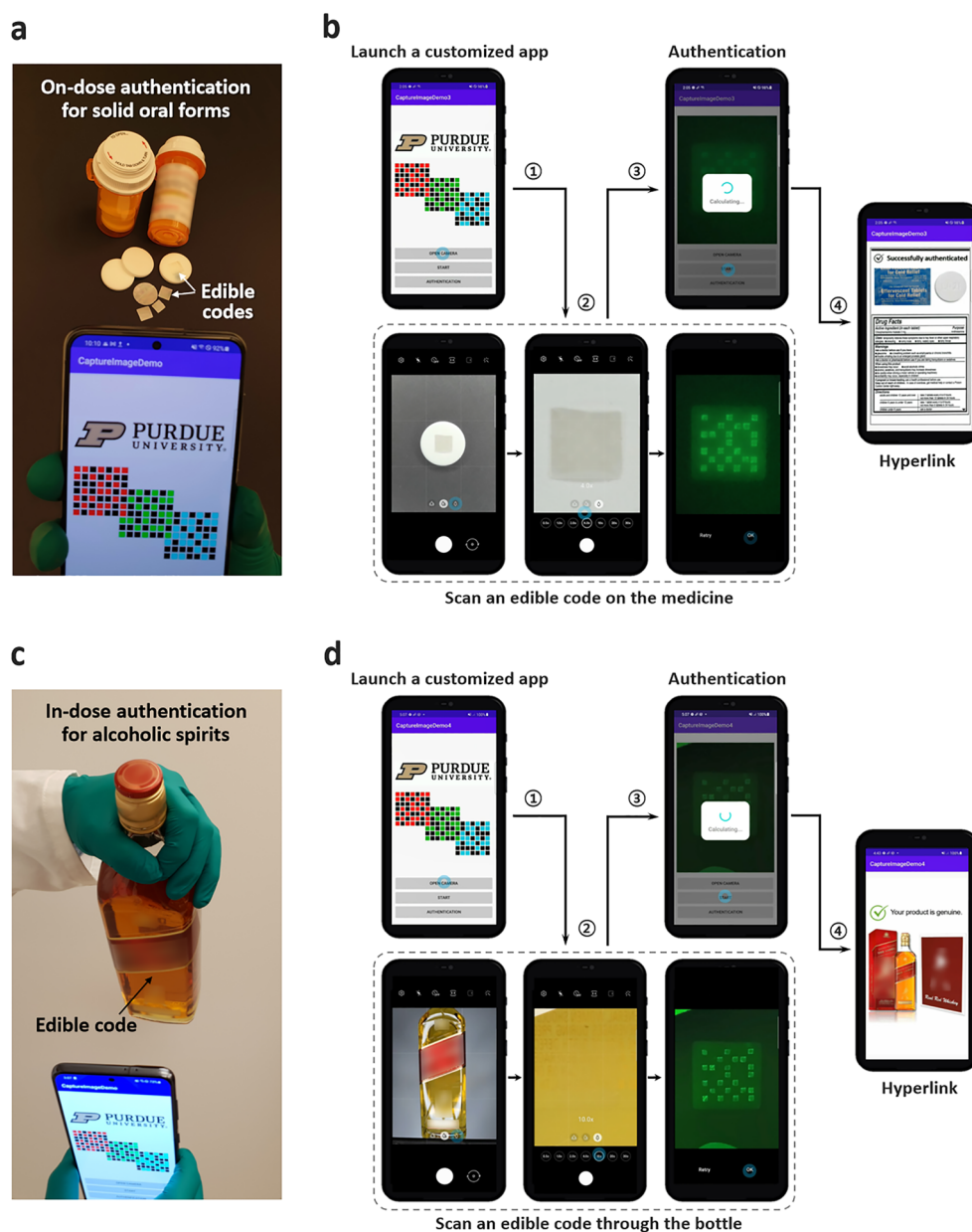
Figure 4. Edible code applications for authentication using a smartphone. (a, b) Simulated on-dose authentication of medicines. (a) Photograph of on-dose authentication of medicines integrated with an edible code. (b) Simulated authentication process for an oral-dosage tablet-type medicine. A custom-built mobile application (app) consists of the following steps for an end user or consumer (Movie S1): launch the customized app, scan an edible code using a set of excitation (470 nm) and emission (525 nm) optical filters (Figure S11). Then, this mobile app authenticates the scanned code and further opens the embedded hyperlink to a webpage to confirm the genuine medicine information, such as product data (e.g., dosage strength, dose frequency, cautions, and expiration date), manufacturing details (e.g., location, date, batch, and lot number), and distribution path (e.g., country, distributor, and wholesaler). (c, d) Bottle-through edible code application for in-dose authentication of high-value alcoholic spirits. (c) Photograph of simulated in-dose authentication of a Scotch whisky bottle (e.g., 80 proof whisky, 40% alcohol per volume) that contains an edible code inside. To image the edible code through the bottle, the bottle is tilted facing down. (d) Simulated authentication process for an alcoholic spirit containing an edible code inside. The customized mobile app can authenticate the scanned code and further inform the genuine product information (Movie S2), such as product data (e.g., type, ingredients, alcohol concentration, and cautions), manufacturing details (e.g., location, date, and serial number), and distribution path (e.g., country, distributor, and wholesaler).
