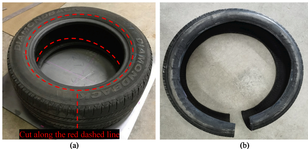
Fig. 3. Method of cutting tyres: (a) cut steel beads and cut cross; (b) cut tyre.
