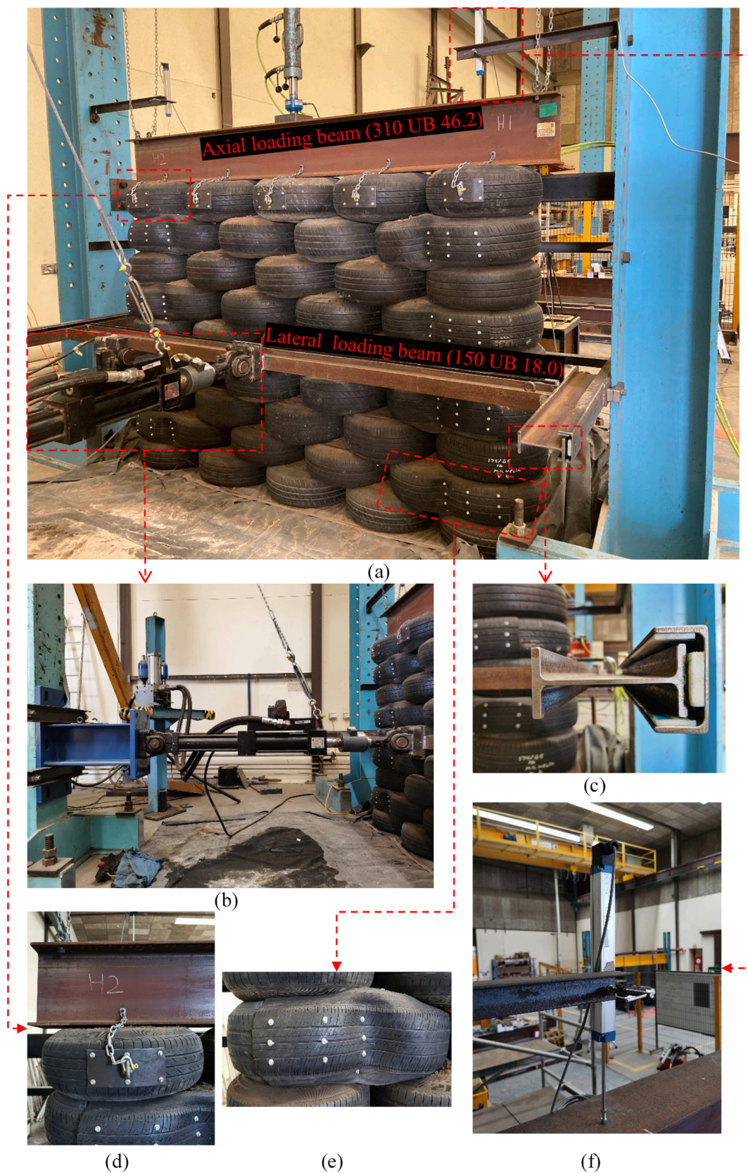
Fig. 5. Front side test setup: (a) overall view; (b) MTS loading machine; (c) lateral loading beam sliding arrangement; (d) safety chain connection between top-course TESEs and axial loading beam; (e) cut tyre connection; (f) Axial LVDT. (Photos b, d, e taken after testing).
