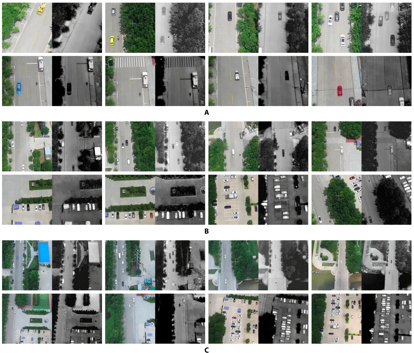
Fig. 5. Some examples of AVIID-3. (A) The height of the UAV is about 50 m. (B) The height of the UAV is about 100 m. (C) The height of the UAV is about 150 m. The AVIID-3 contains various scenes with complicated background, including roads, bridges, parking lots, and streets, and the number of images of each scene are 938, 134, 158, and 50, respectively.
