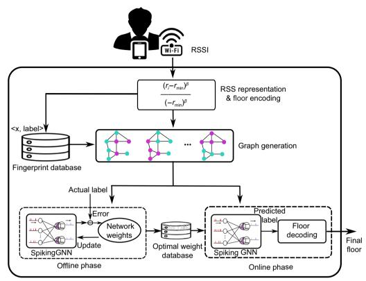
Fig. 1 Overview of *FloorLocator*. It takes as input WiFi scans, which are organized in a graph of visible APs before feeding into a spiking graph neural network for training and predicting. Each module of *FloorLocator* will be detailed in Section V
